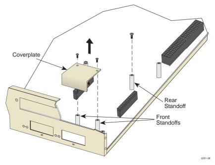
Figure C-4 Coverplate Removal
